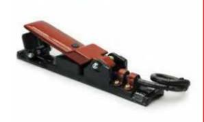
**RAV Electric.**When using blast hoses over 40 meters long the RAV Electric remote handle will provide instant activation of the pot remote valve and eliminate the delay encountered with pneumatic handles. The handle operates on 12VDC supply.
