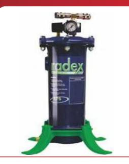
Radex Breathing Air Filter. The Radex Airline Filter System offers more capacity, more filtration and more vesatility. Can be floor or wall mounted with same mounting bracket. Large capacity 6 stage filter cartridge removes moisture and particulates to 0.5 micron and odor from the compressed air providing the operator with clean breathable air. Large range of optional equipment allows the filter to be configured to met specific breathing air requirements.
