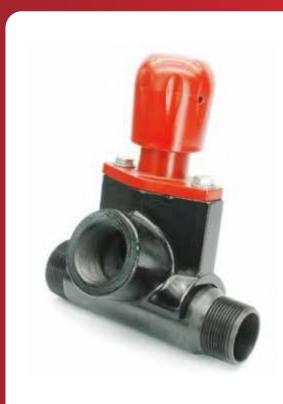
**Abrasive Saver Valve.** Reduce abrasive consumption and save money. The alpha-blast Abrasive Saver Valve will save a fortune in wasted abrasive. The screw in plunger permits very accurate adjustment to allow just the right amount of abrasive to the blast nozzle.
