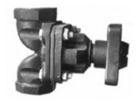
**Isolator Valve.** The alpha-blast Isolator Valve is a great maintenance time saving device. Fitted above the abrasive metering valve it permits the metering valve to be removed from the blast pot for service, without the need to empty the abrasive from the pot, which saves a huge amount of time.
