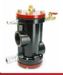
**RAV125 Inlet Valve.** The blasting industries favourite remote control valve. Simple springless design ensures continuous reliable service for thousands of cycles. Removable end caps provides quick and simple access to the valve interior for servicing. Fitment of mini ball valve allows the valve to be deactivated in case of emergency.
