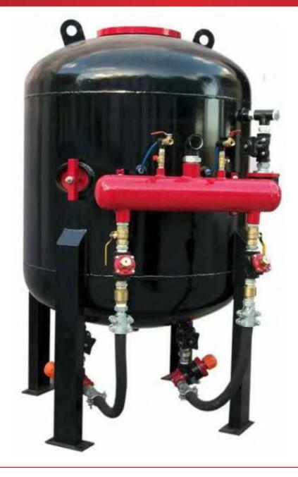
**FatBoy Blasting Pot.** The alpha-blast FatBoy range of blast pots have been developed specifically to increase blasting productivity in open blast work sites using consumable abrasives. Available in three standard sizes, the FatBoy blasting pots are sized for 1, 2 or 4 metric tonnes of garnet abrasive. The pressure hold design of the system allows each operator to have independent control for starting and stopping blasting. An abrasive blow down function may also be incorporated if required.
