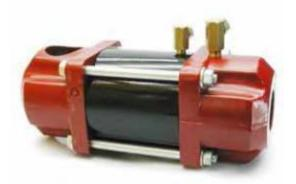
**Combination Valve.** This valve is a one piece normally closed air inlet and outlet valve. A short length of blast hose is used for the blow down function that eliminates any abrasive coming into contact with the valve. As no abrasive passes through the valve there is no wear on the valve thus providing years of trouble free service.
