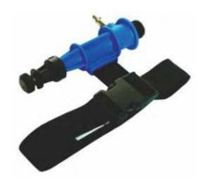
**Cold Air Tube.**The Cold Air Tube Assembly cools compressed breathing air coming into respirators by as much as 32°F (18°C). The Cold Air Tube helps to maximise worker comfort and increase productivity whilst working in hot climates. The Cold Air Tube is fitted with an airflow regulator which allows the user to adjust the outgoing air temperature.
