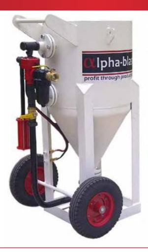
**SuperFlow Design.** Conventional blast pots are fitted with 90 degree lower cone. The SuperFlow design is 120 degree steep lower cone. This increased angle of the lower cone provides a more consistent abrasive flow to the metering valve and ensures the pot is suitable for all abrasive types. Even the finest of abrasives ie, garnet, glass beads, sodium bicarbonate etc, will flow smoothly and uninterrupted.
