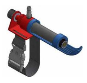
**Aluminium Cool Air Tube.** The alpha-blast aluminium air cooler is used to cool the incoming hot air supply from the compressor prior to it entering the helmet. The cooler will reduce the temperature of the incoming air supply up to 32°F (18°C). This cooler incoming air ensures maximum operator comfort in hot climates. When the blaster is comfortable productivity increases.
