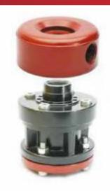
**RAV125 Outlet Valve.** The blasting industries favourite remote control valve. Simple springless design ensures continuous reliable service for thousands of cycles. Removable end caps provides quick and simple access to the valve interior for servicing. Exhaust air noise is greatly reduced by fitment of silencer to top cover.
