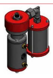
RAV50 Mini Combination Inlet/Outlet Valve. The RAV50 Mini Combination Valve allows for ease of installation and maintenance with only one valve requiring removal for quick change over of respective diaphragms, gaskets and o rings, meaning down time is kept to an absolute minimum. Supplied complete with exhaust silencer.
