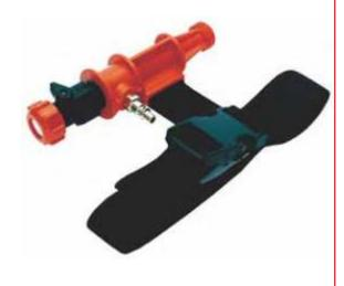
Hot Air Tube. The Hot Air Tube Assembly warms compressed breathing air coming into respirators by as much as 30°F (17°C). The Hot Air Tube helps to maximise worker comfort and increase productivity whilst working in cold climates. The Hot Air Tube is fitted with an airflow regulator which allows the user to adjust the outgoing air temperature.
