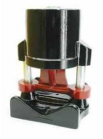
**Pinch Valve.** Tough, simple and reliable the alpha-blast Pinch Valve is used to shut off abrasive and air flow in the blast hose as it leaves the abrasive metering valve. Simple pneumatic operation and minimal moving parts ensure reliable continuous operation.
