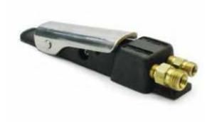
**CRV Pneumatic.** This nonair bleed type deadman handle is recommended for use with the Combination Valve. The internal 3 way normally closed valve provides a fast activation and deactivation response time.
